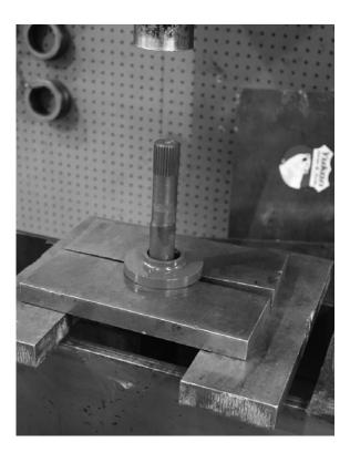
If using a press, place the axle puller body & axle into the press. The top lip of the puller body is supported by the press plates. Make sure you have enough room between the bottom of the axle and the floor for bearing removal before operating the press.
