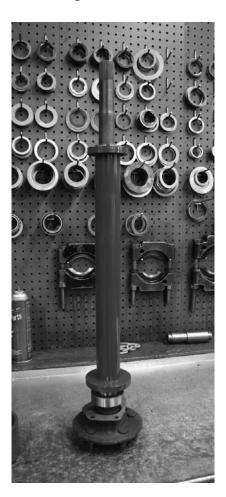
Begin by sliding the body of the puller over the axle shaft and seating it against the bearing.
