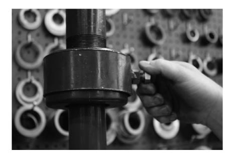
Slide the retaining sleeve over the clamshells. Tighten down the retaining bolt to secure the retainer and clamshells in place.
