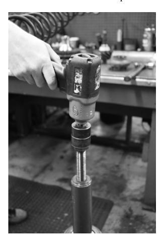
Use an air impact gun to complete the bearing removal.
