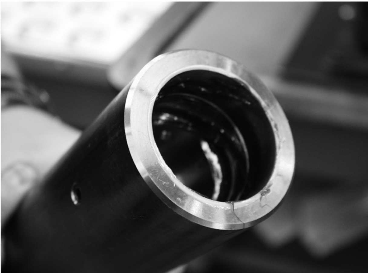
Apply a liberal amount of bearing grease to the boring tool threads.
