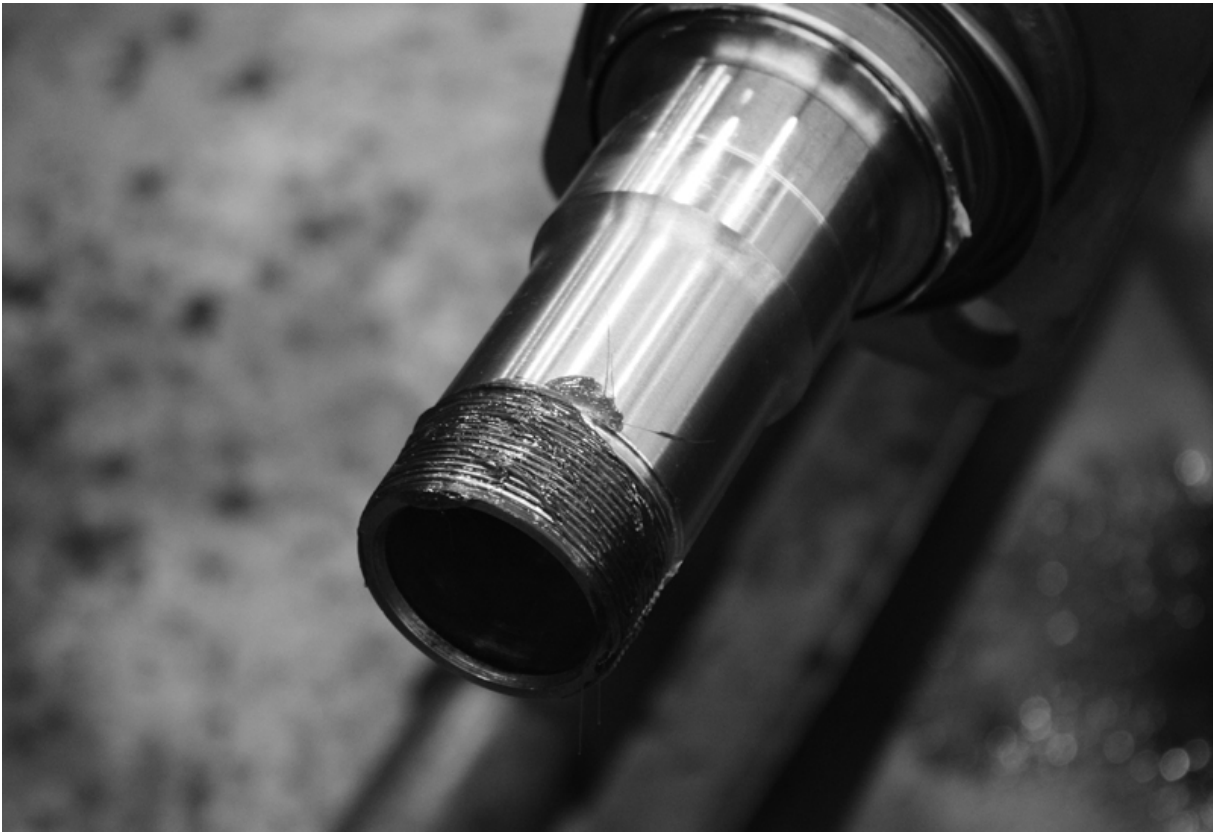
Apply a liberal amount of bearing grease to the spindle threads.
