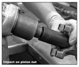
bearings will have a long life. If the crush sleeve is over crushed and the pinion bearing preload exceeds the specified allowable range the only solution that I know of is to install another new crush sleeve and start over. After reaching the correct preload, I moderately tap both ends of the pinion to seat the bearings, races and yoke. Be careful not to hit the pinion so hard that it damages the bearings. After "seating" the pinion, I check the preload again to make certain that it is correct.
