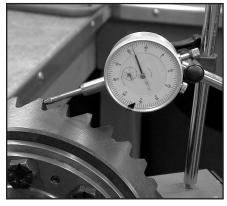
This is accomplished by a preload shim pack (of various thicknesses) or a collapsible crush sleeve. A new crush sleeve should always be used during final assembly.
