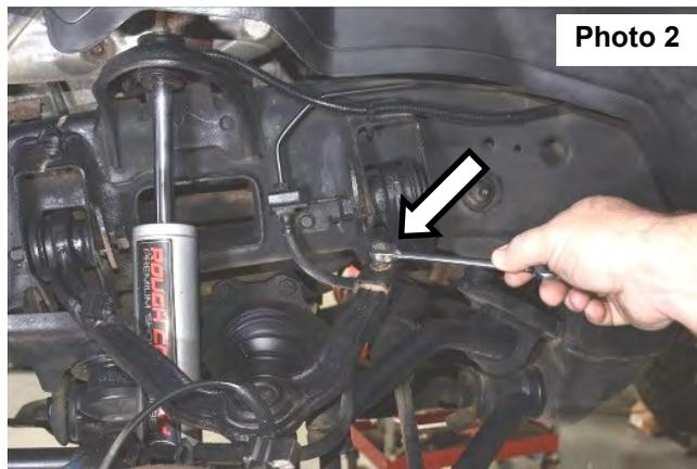
6. Remove and unplug the ABS sensor wire from the frame.
