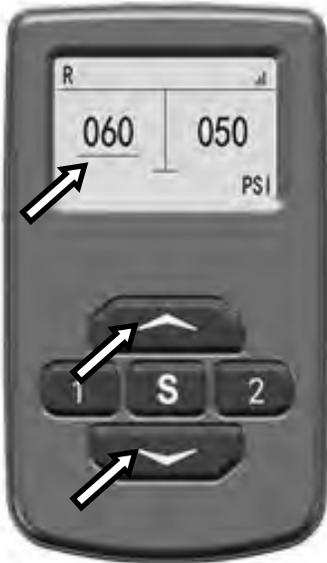
Confirm CH-1/CH-2 on the screen to confirm whether the current status is Channel 1 or Channel 2. The status shown in the figure is Channel 1 in the status shown in the figure.
