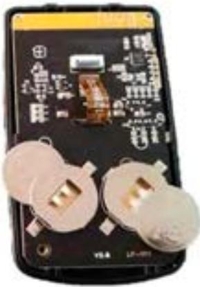
Install qty 2 of the CR2032 batteries as shown. Pay attention to the positive and negative terminals of the battery.
