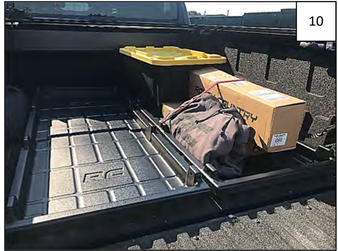
Slide tray back to close tail gate – tightened straps will keep tray from moving further into bed.
