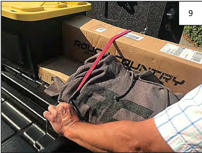
Use bungee cords (not provided) to secure items being stored in tray. Insert hooks through slots around perimeter of Bed Storage Tray. Criss Cross bungee cords to secure items.
