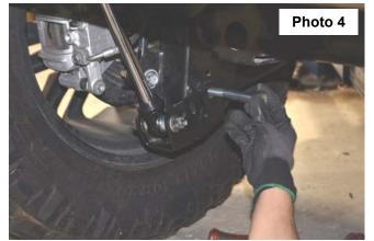
Using an 18mm wrench and socket, torque the lower shock mount bolt to the factory spec. Using a 21mm socket and wrench, torque the lower control arm bolt to 120ft/ lbs. See Photo 5.
