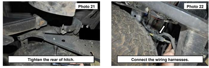
22. Reconnect the rear license plate light and proximity sensor wiring harness. See Photo 22.
