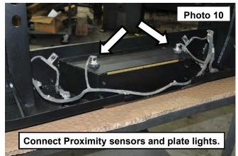
Secure the wiring harness along the bumper using the supplied wire ties.
