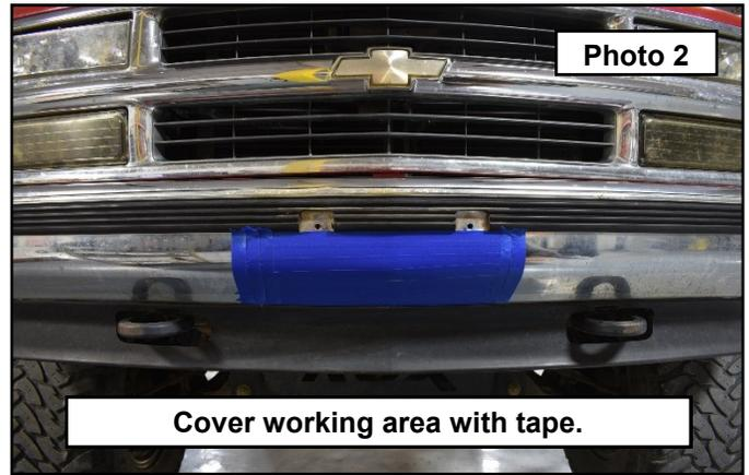
4. Cut out the template halves from the instruction booklet and tape together. Tape to the bumper using the valance as a guide if vehicle has one. If vehicle is missing the valance, use the straight edge of the template and tape to the bumper 1" from the back edge. Mark around the template. This is only a guide and may need more cutting, grinding, and/or sanding for a clean, flush look. So cut to the inside of the lines made. **Photo 3**
