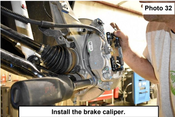
Install the brake caliper.
