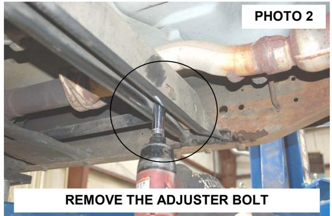
4. The next step will require a torsion bar tool to safely unload the torsion bars. Part # 1067 is available from Rough Country. **Please Note the torsion bar is under extreme load. Substituting a tool for an actual torsion bar tool may result in injury.**
