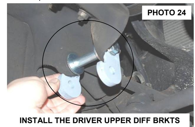
32. Raise the differential and install it in the upper driver bracket with the supplied 9/16" x 5" bolt, washers and nut. Also install the differential in the passenger side with the factory hardware. Do not fully tighten at this time.
