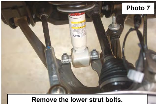
**Remove the lower strut bolts.**
