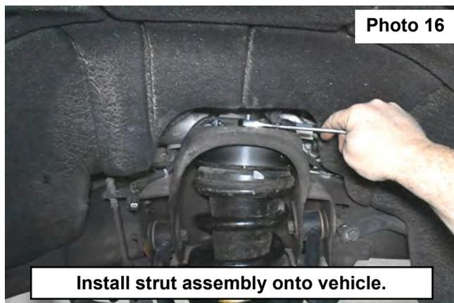
22. Install the strut in the lower control arm using supplied 3/8" x 2.25" bolts, washers, and nuts. **See Photo 17.** It may be necessary to jack up the lower control arm with a floor jack to align lower strut holes.
