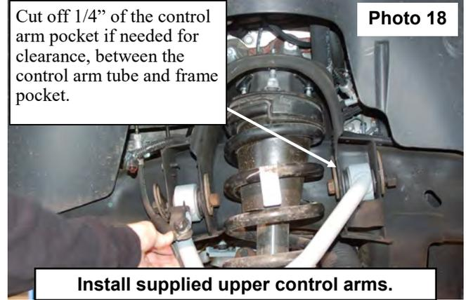
24. Install the supplied control arm with factory hardware. Reinstall the knuckle to the upper control arm with the supplied castle nuts/cotter pins. Tighten using 3/4" wrench to **50 ft/lbs. DO NOT OVER-TORQUE THE CASTLE NUT.** Reinstall the tie rod end into the knuckle with factory hardware and using a 21mm wrench.
