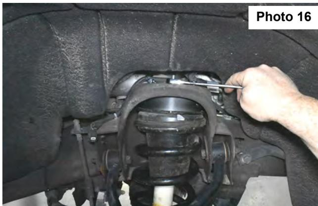
22. Install the strut in the lower control arm using supplied 3/8" x 2.25" bolts, washers, and nuts. **See Photo 17.** It may be necessary to jack up the lower control arm with a floor jack to align lower strut holes.
