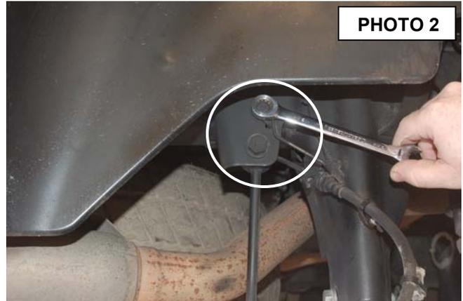
4. Remove sway-bar link using 8mm and 18mm wrench for lower end and 18mm for top end. **See Photo 3 & 4.**
