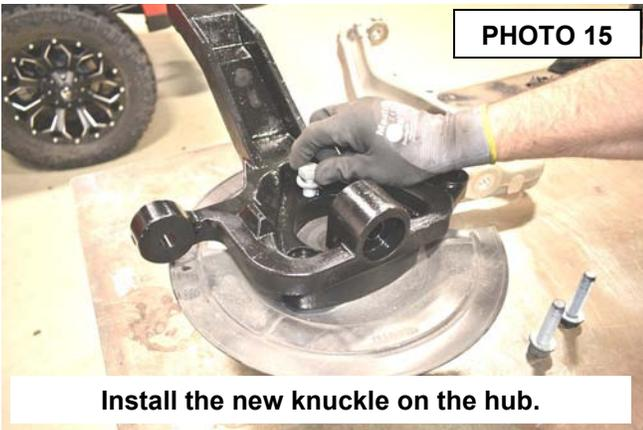
**Install the new knuckle on the hub.**
