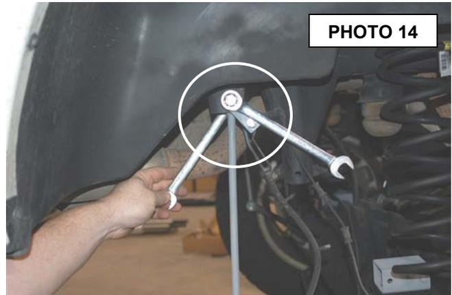
20. Use a 18mm and 19 mm to tighten sway bar link bolts and 13 mm for brake line bolts.
