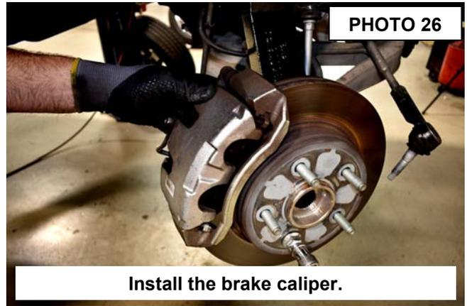
31. Torque the brake caliper bolts to factory specs using a 21mm socket. **See Photos 27 & 28.**
