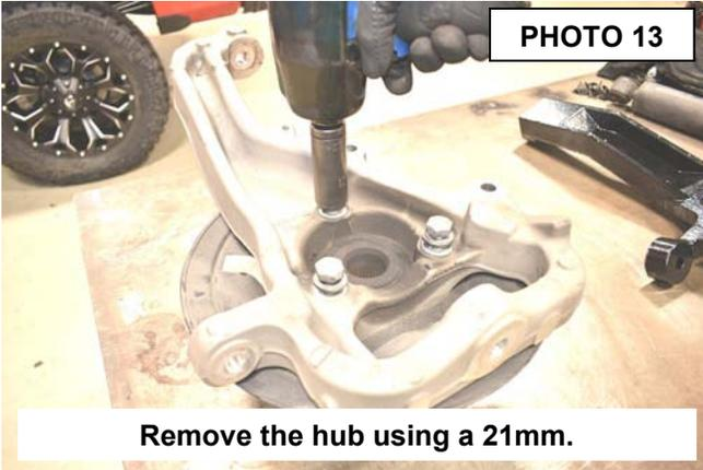
**Remove the hub using a 21mm.**
