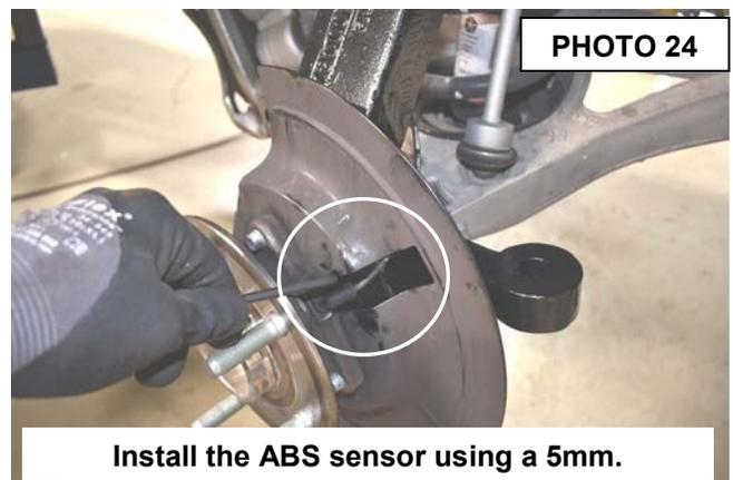
**Install the ABS sensor using a 5mm.**
