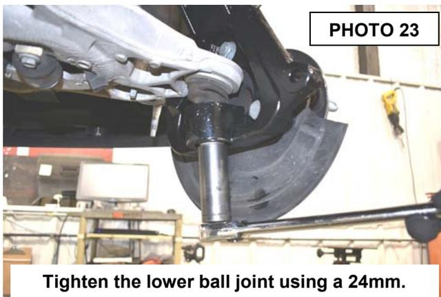
**Tighten the lower ball joint using a 24mm.**
