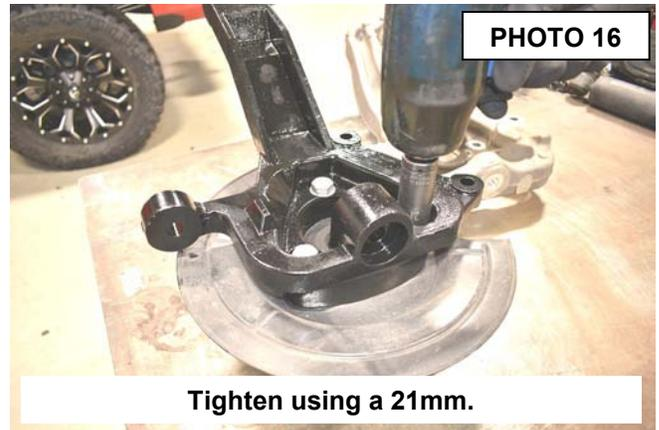
**Tighten using a 21mm.**
