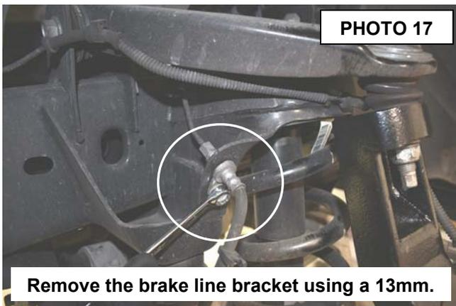
**Remove the brake line bracket using a 13mm.**
