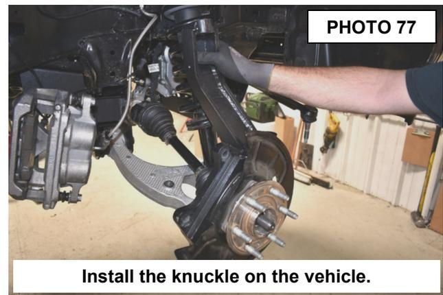
**Install the knuckle on the vehicle.**
