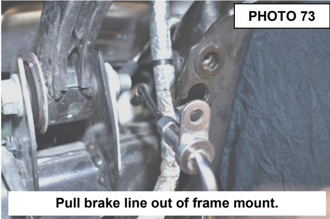
**Pull brake line out of frame mount.**
