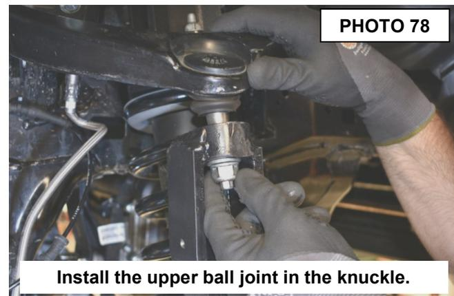
**Install the upper ball joint in the knuckle.**
