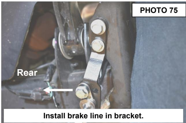
**Install brake line in bracket.**
