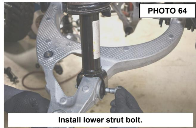
71. Install the factory hardware into the lower mount. Do not tighten at this time. See **Photo 64.**
