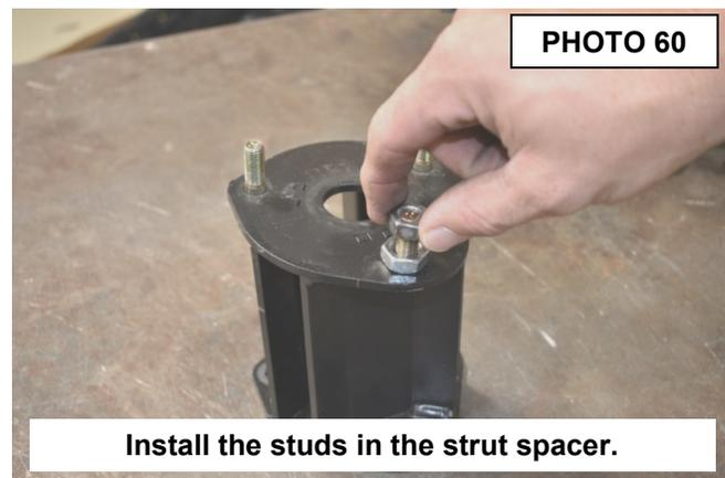
68. Using a 17mm wrench, tighten the 10mm nut to pull the stud into the spacer. **Do not use an impact.** See **Photo 61.**
