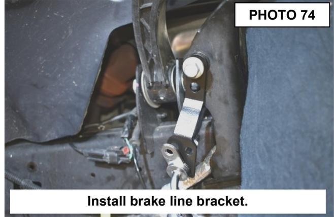
**Install brake line bracket.**
