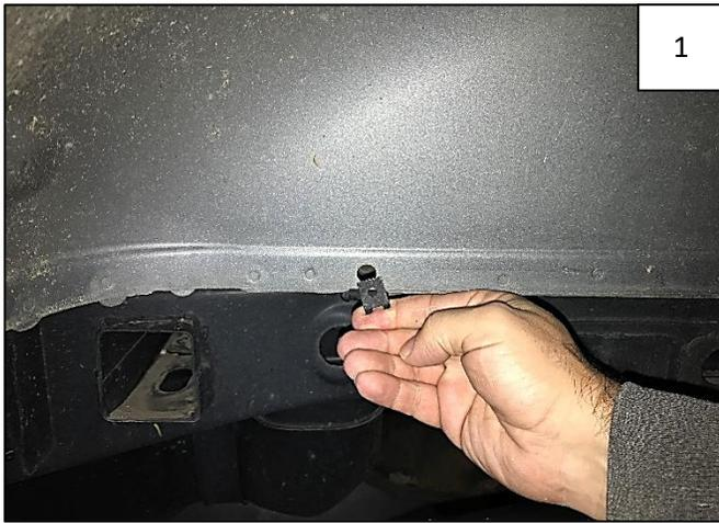
Install 2 supplied "U" Clips over factory holes at back of rear wheel well, as indicated in next step. Flat side of clip will face *out* when clip is installed.
