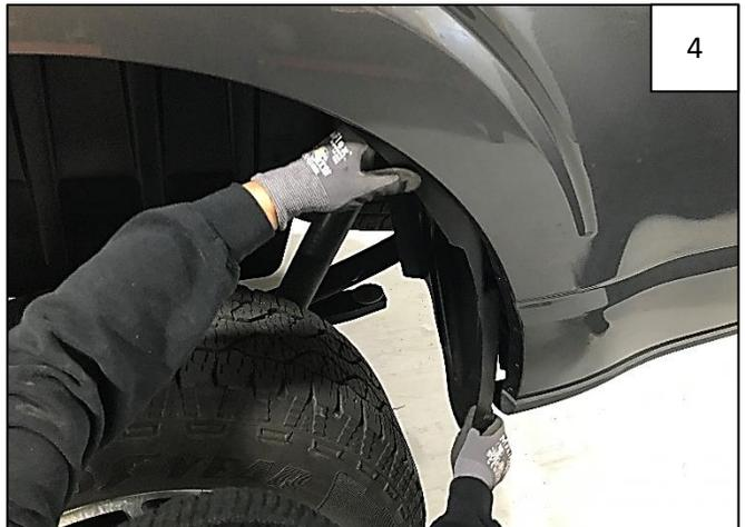
Tuck Rear Wheel Well Liner behind sheet metal at lower edges, and under metal fender lip at all other outward facing edges.
