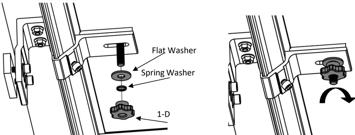
※ATTENTION: Make sure the Flat Washer and Spring Washer are all placed on bolt before screw the plastic nut on.
