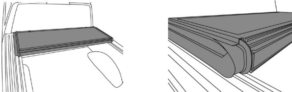
8. Adjust the front support plate(1-F) to correct position, insert the front bolt with rubber washer into the holes on the cover front panel and front support plate. Then tighten the hand nut under the front support plate.
