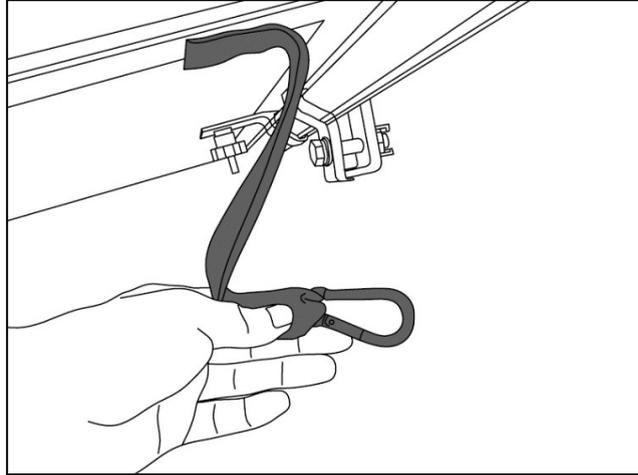
**When installing the side rail, make sure one side rail clamp (2-G) is installed nearby the Strap Safety Buckle position.**
