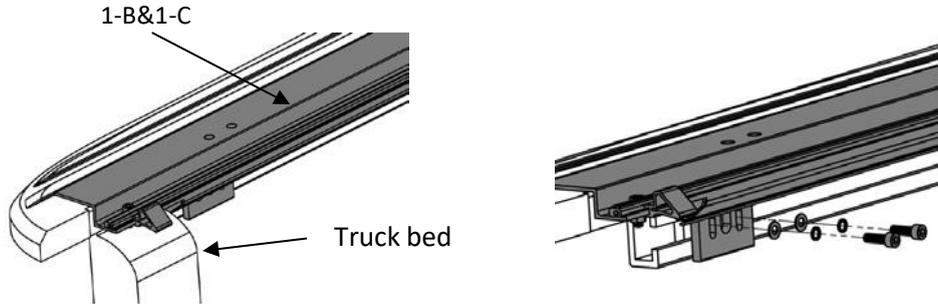
7. Place the bed cover on the front end of truck bed. Ensure the cover is even on all sides and sit firmly on side rails.
