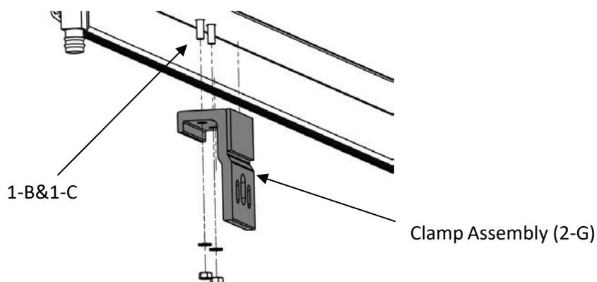
Step-3 Place the side rail on the bed rail, and push it to the front wall of truck bed. Place one clamp at the front of the side rail and one at the rear (please make sure the rear clamps is placed on the position that is closest to tailgate). Tighten the clamps each side.
