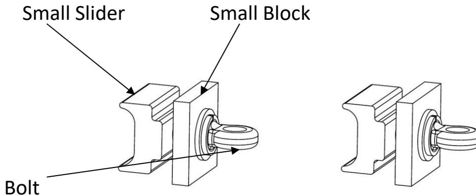
**Insert the small slider into the Track Channel. Tighten the bolt. (Note: Make sure the small slider is installed nearby the Strap Safety Buckle position) There is a hole on the bottom of the bolt. Snap the safety buckle into the hole of the bolt.**
