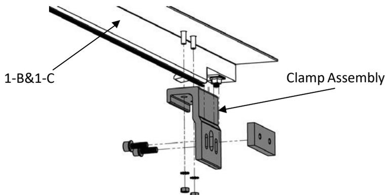
Step-2 Attach and Install the other set of Clamp Assembly (2-G) to the Side Rail (1-B&1-C), then tighten the nuts.
