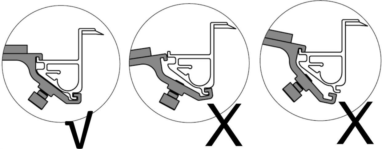
2-2 Slide the Side Rail Locking Latch (1-G) into side rail (from rear end) and move it to the rear part of side rail. Do not tighten the bolts.
