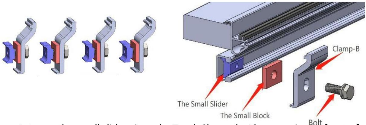
Step-1. Insert the small sliders into the Track Channels. Place one in the front of channel and the other one in the rear of the channel. \*For 6.5' bed, an additional slider will install in the middle of channel.
