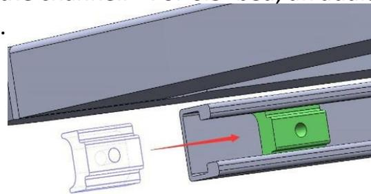
Step-2. Secure the side rail and truck bed with the clamps (Bolt the Clamp-B, the small Block and the Small Slider together). Place one clamp at the front of the side rail and one at the most rear position. Tighten the clamps each side. Then follow the main Installation. \*For 6.5' beds, an additional slider will be installed in the middle of side rail.
