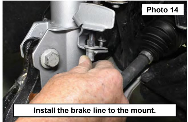
14. Attach the ABS line to the strut mount and the clip installed in the mounting hole. **See Photo 15.**
