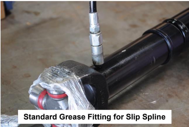
**Standard Grease Fitting for Slip Spline**
