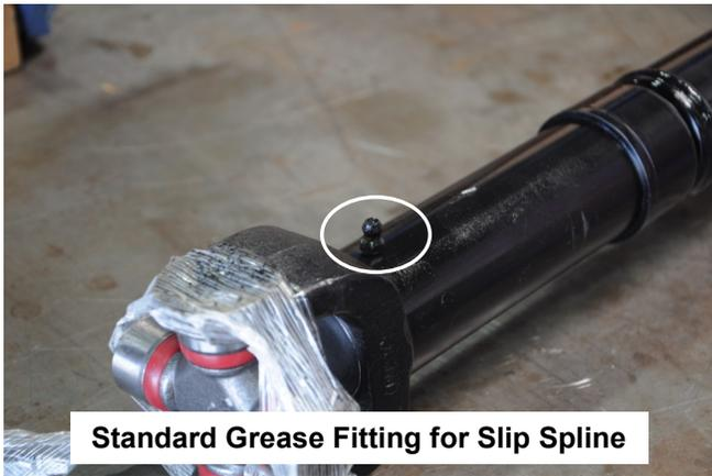
**Standard Grease Fitting for Slip Spline**
