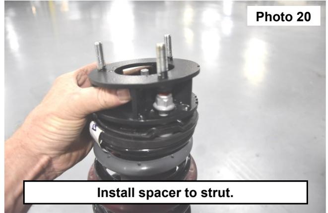
19. Reinstall the upper strut with the spacer to the vehicle with the supplied 10mm flange nuts using a 16mm socket/wrench. **See Photo 21.**
