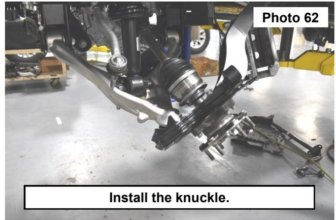
60. Install the knuckle to the upper ball joint using the stock hardware. **See Photo 64.**
