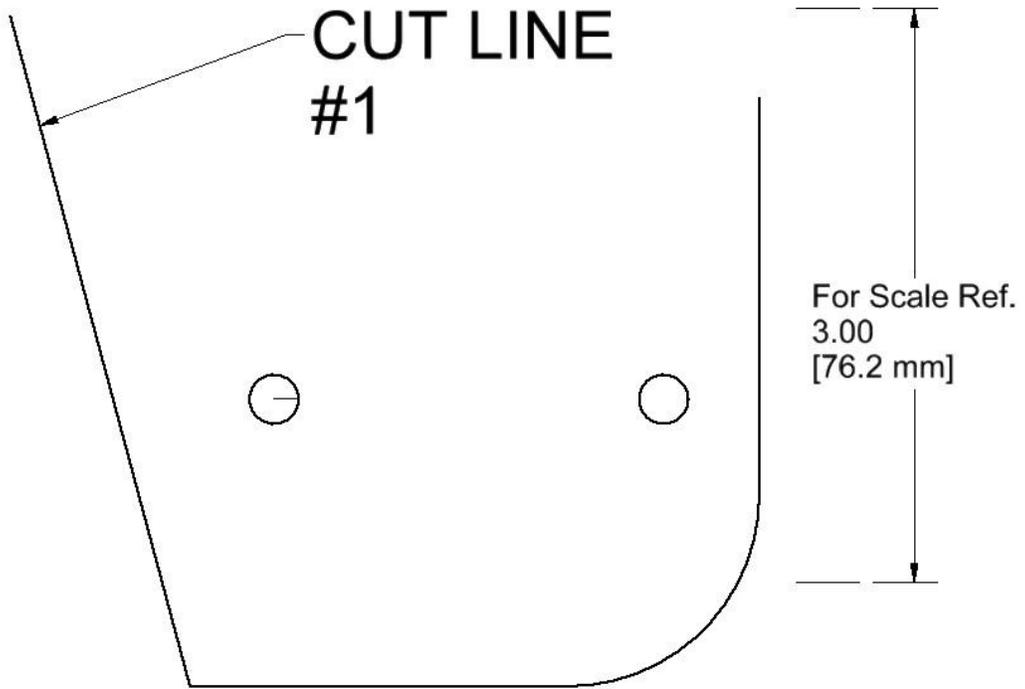
Mark at arrows when template is on the vehicle.
