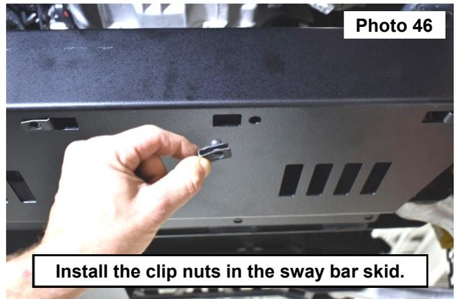
**Install the clip nuts in the sway bar skid.**
