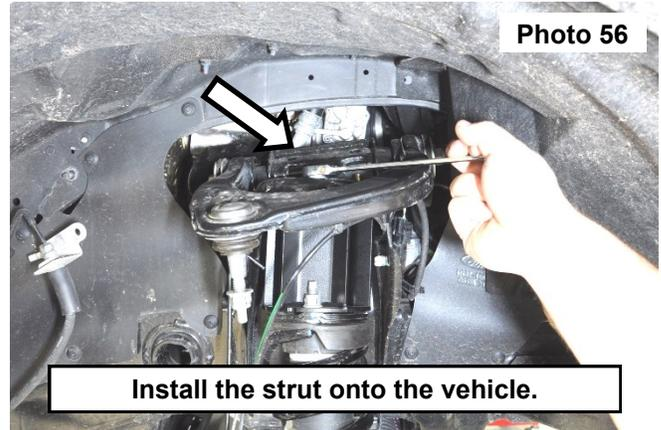
54. Raise the lower control arm up and install the lower strut to the control arm using the stock hardware. **See Photo 57.**
