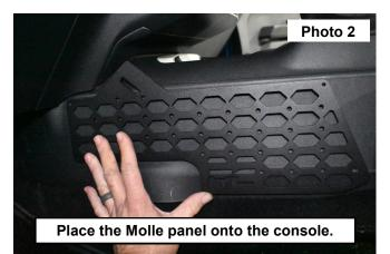
Place (2) of the spacers in-between the molle panel and the console on the upper two mounting holes. See Photo 3.
