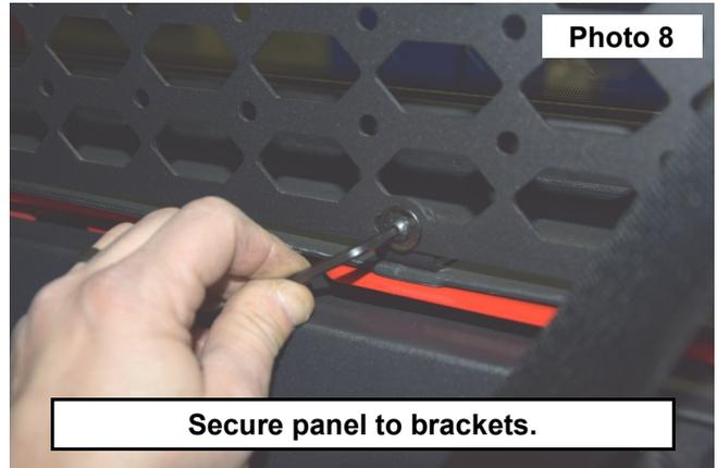
**▲ NOTICE** In order to remove the roof again, the L-brackets and accompanying hardware will need to be removed. With the roof off, hardware can be reinstalled with all bolt heads facing out.
