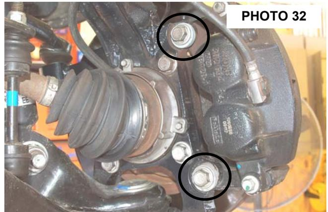
43. Make sure the vacuum hose and ABS wire are out of harms way. Using the supplied zip tie, secure the vacuum hose and ABS wire to the knuckle neck.
