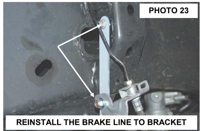
30. On the driver side, pull slightly on the brake line to allow the line to be installed on the new bracket. Secure the brake line to the new bracket with the supplied 5/16" x 3/4" bolt, washers and nut.
