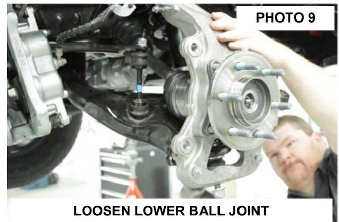
13. Remove the upper and lower ball joint nuts and remove the knuckle from the vehicle.
