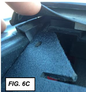
Another way to set the tailgate cap seals is to use the Tailgate Seal Gauge as shown in figure 6B & 6C. You should be able to just slide the Tailgate Seal Gauge in between the Tailgate Cap Seal and the Bottom Cap.
