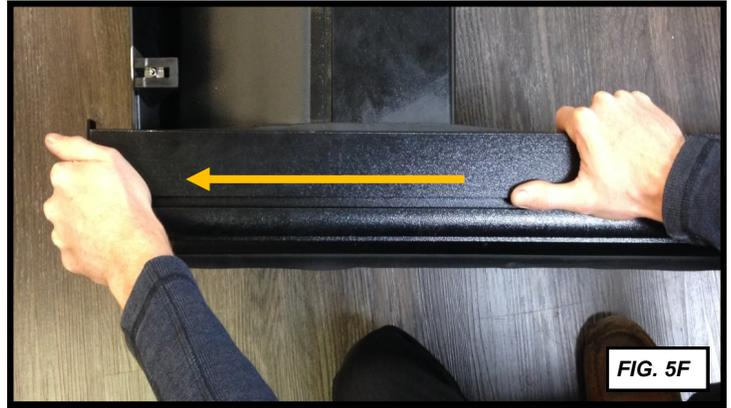
Then you can thread the Lead Rib into the rail and push the rail forward to the end of the can (FIG 5E & 5F). If you have difficulty threading the Lead Rib into the rail, you can gently lift up on the lead rib with your left hand while pushing the rail forward with your right. Next push the cab caps into the front of the rails (FIG 5G). Finally secure the rail to the canister with the Rail Screws provided with flat washer and lock washer (FIG 5H).
