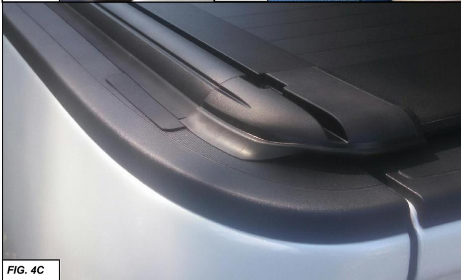
Included with your tonneau cover is a stake pocket cover. This helps to trim the outside seal for your rails (*FIG. 4C*). First clean the stake pocket hole area. If you have Isopropyl Alcohol this will work well. After the stake pocket area is dry peel off the adhesive backing and stick the cover on the hole so that it is entirely covered (*FIG 4A & 4B*).
