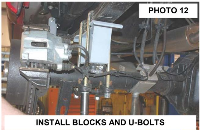
14. Install the upper leaf spring u-bolts on leaf spring and blocks. Secure with supplied u-bolts and tighten using a 16mm socket. **See Photo 12.**
