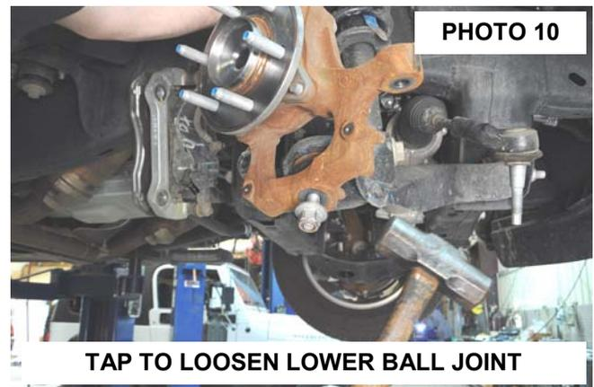
13. Remove the upper and lower ball joint nuts and remove the knuckle from the vehicle.
