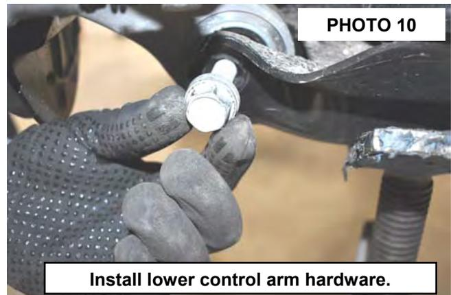
12. Using an 18mm wrench and socket, torque the lower control arm bolt to factory specs. **See Photo 11.**
