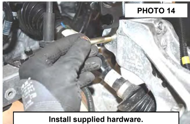
17. Install the sway link using the factory hardware and tighten using a 5mm Allen and 15mm wrench.
