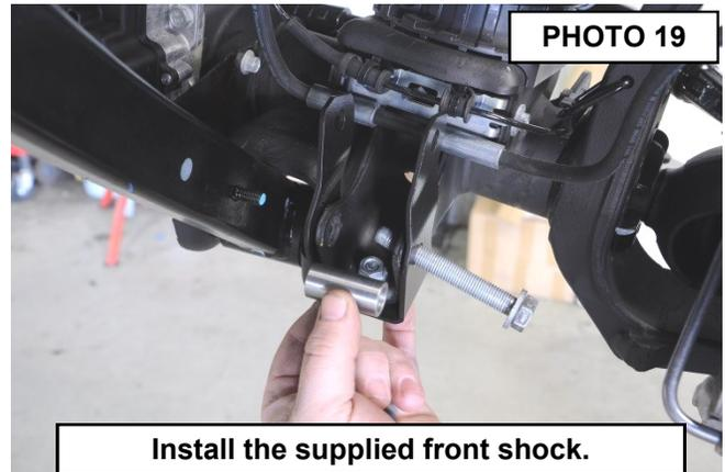
24. Using a jack to compress the suspension, install the shock in the extension bracket using the supplied 12mm x 65mm bolt, 1/2" washers, and 12mm nut (1676BAG). **See Photo 20.** Tighten the factory bolt using an 18mm socket and wrench. Torque to 55ft/lbs. Tighten the lower shock bolt using an 18mm socket and wrench. Torque to 55ft/lbs.
