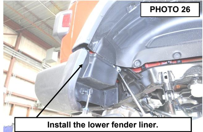
26. Install the lower fender liner using the stock hardware, tighten using an 8mm socket. **See Photo 26.**
