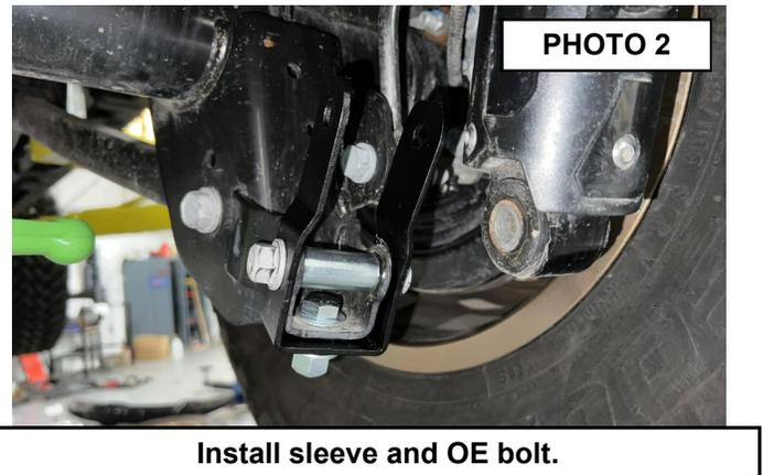
3. Attach the shock to the shock relocation bracket using the supplied 12mm x 65mm bolt and flange lock nut (60600BAG1). **Do not tighten at this time. See Photo 3.**
