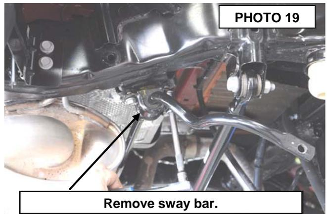
23. **▲ NOTICE** Flip the sway bar from passenger side to driver side.
