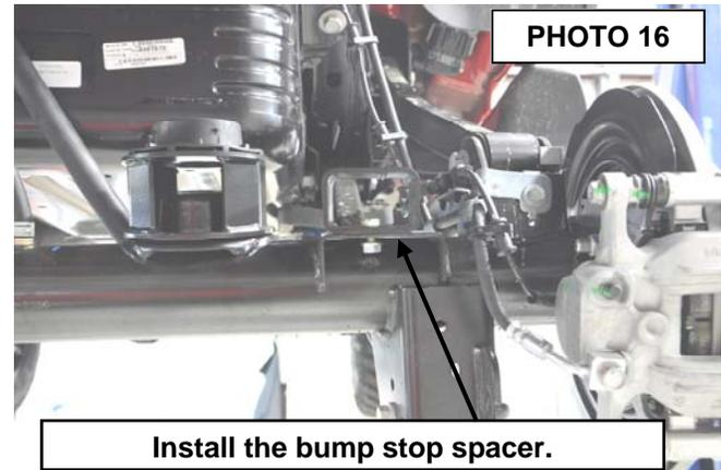
19. Install the supplied bump stop spacer on the axle using the supplied 3/8" x .75" bolts, washers, and flange lock nuts. (You will use 2 bolts, 2 washers, and 2 nuts per side). Using a 9/16" wrench and socket, torque the hardware to 30ft/lbs. **See Photos 16 & 17.**
