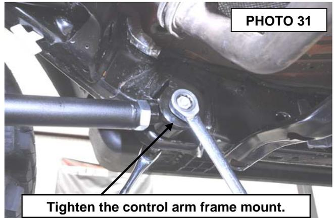
**Tighten the control arm frame mount.**
