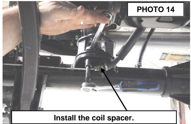
17. Install the coil spring spacer on the axle using the supplied 3/8" x 1" bolt and flange lock nut (65430BAG2). Torque to 30ft/lbs using a 9/16" wrench and socket. **See Photo 14.**
