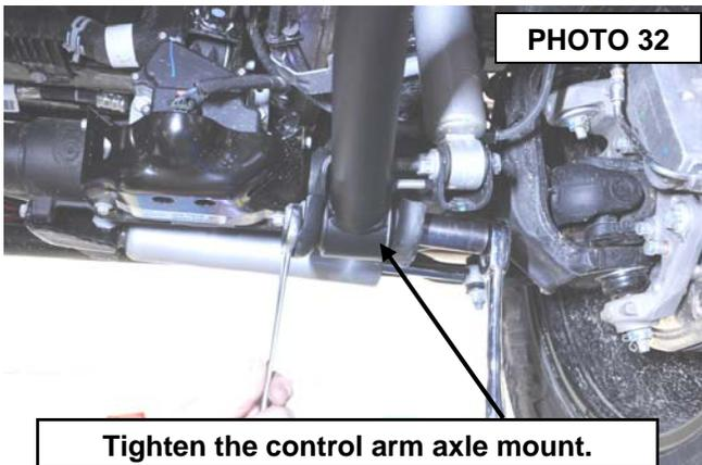
**Tighten the control arm axle mount.**
