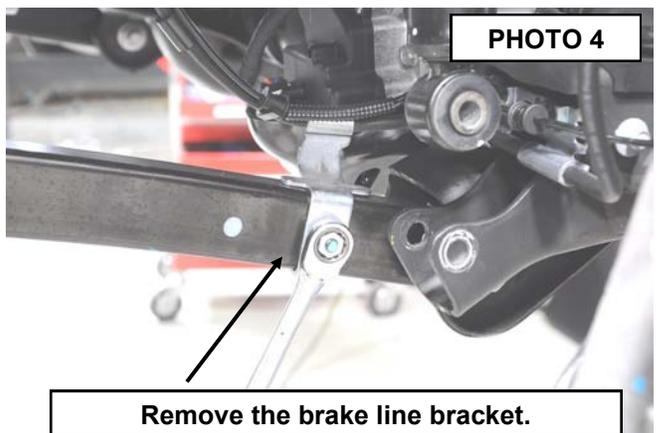
7. Using a 15mm wrench, remove the brake line bracket from the lower control arm. **See Photos 4 & 5.** Retain hardware for reuse.
