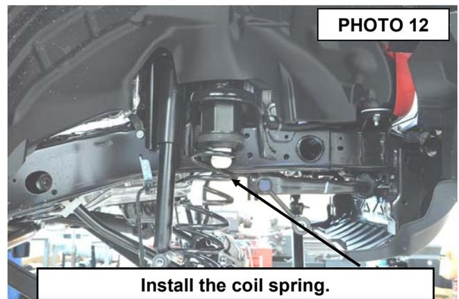
15. Install the bump stop spacer into the lower coil mount. **See Photo 12.**
