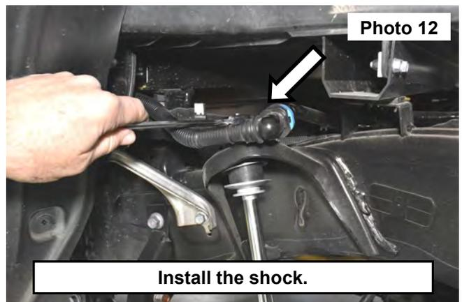
14. Install the lower shock end on to the axle mount, then secure using the OE bolt. **See Photo 13.**
