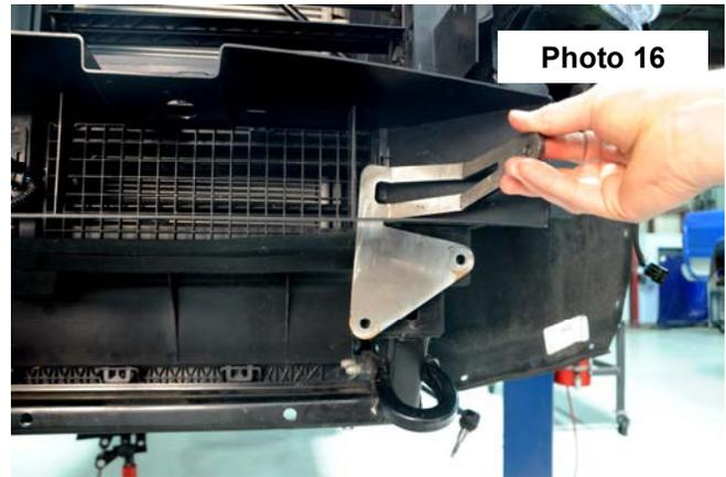
16. Using factory hardware, install crash bar in factory location and tighten with a 15mm socket. **See Photo 17.**
