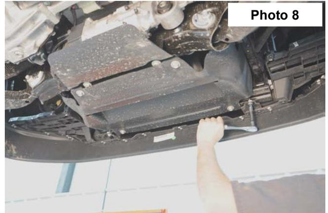
11. Remove the 4 bolts holding the crash bar to the frame with a 15mm socket . **See Photo 9.**
