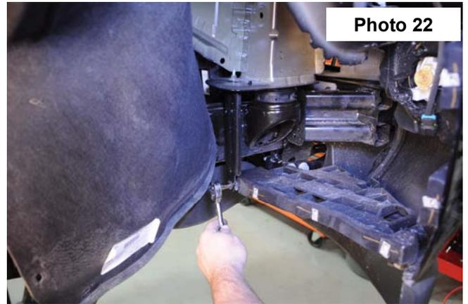
22. Attach the inner fender with the factory fender screws and push pins. Tighten with a T15 torx bit. **See Photo 23.**
