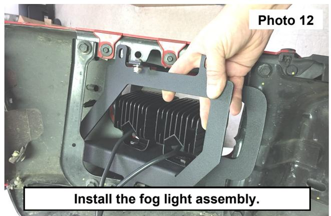
14. Install the fog light assembly into the front bumper. **See Photo 12.**
