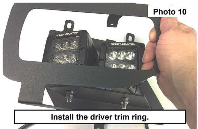
ers and (2) 1/4-20 nylock nuts. Tighten using a 3/16 Allen wrench and a 7/16" wrench. **See Photo 10 and 11.**
