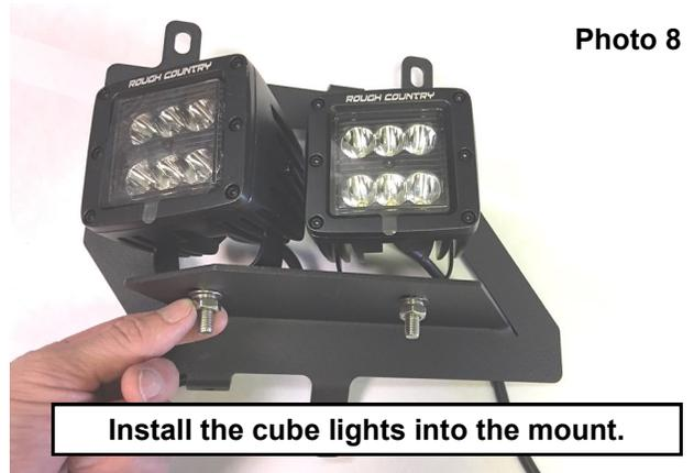
11. Install the (2) cube lights into the mount using the supplied hardware in the LED cube light kit. **See Photo 8.**
