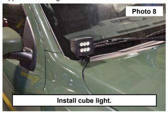
8. Run the wiring as desired and be sure to keep away from moving parts and hot surfaces.
