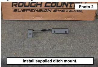
Slowly lower the hood until the ditch mount comes into contact with the cowl and trace around the ditch mount.
