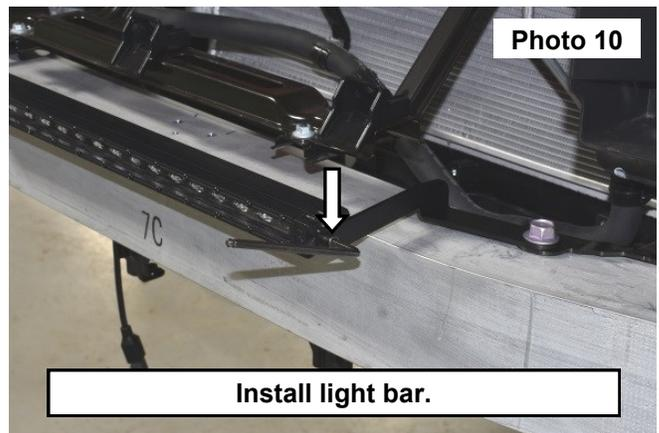
10. Run the light bar wiring as desired to the power source. Be sure to keep away from hot or moving parts.
