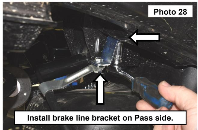
shaft with the stock bolts at the frame and the supplied 5/16" x 3/4" bolts, washer, and nut at the brake lines using 1/2" socket/wrench. **See Photo 28, 29, 30, and 31.**
