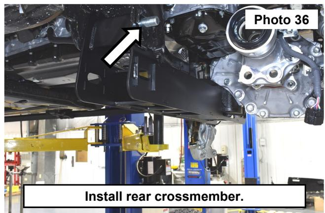
36. Secure the diff to the rear crossmember using the stock hardware. See Photo 37 and Photo 38.
