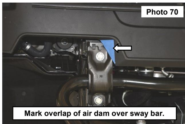
69. Trim the overlapped area on the air dam, Shown clearing the sway bar drop. **See Photo 71.**
