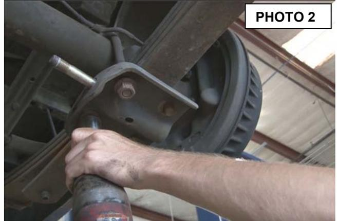
5. Raise the rear axle and install the new supplied block between the axle and the leaf spring. Make sure the smaller end of the block points to the front of the truck. **See Photo 3.**
