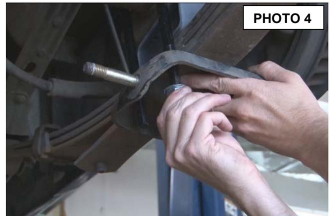
7. Install the lower mount of the rear factory shock to the u-bolt plate using factory hardware and a 21mm socket.
