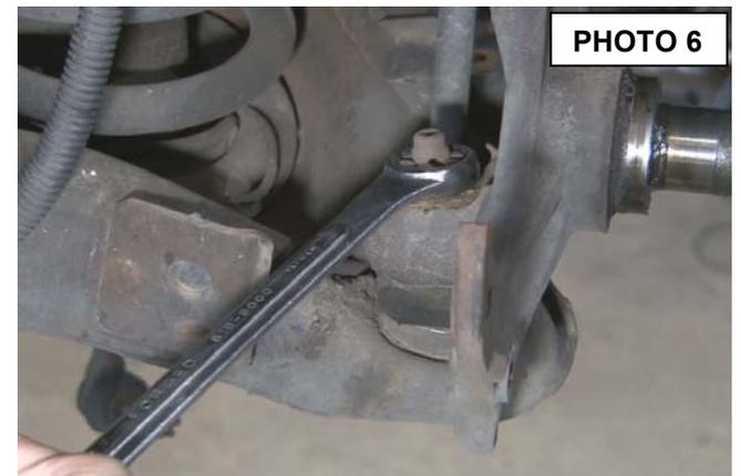
9. Remove the upper ball joint cotter pin and then loosen the upper ball joint nut using a 15/16" wrench as shown in **Photo 7**. Do not remove nut.
