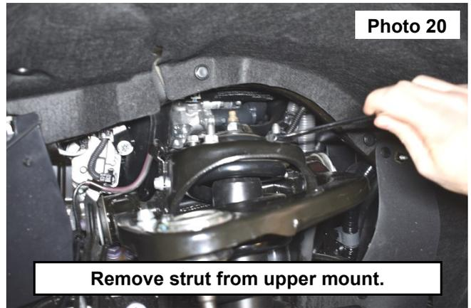
20. Loosen lower control arm cam bolts using two 24mm sockets/wrenches to allow the lower control arm to drop and remove the strut from the vehicle. **See Photo 21.**
