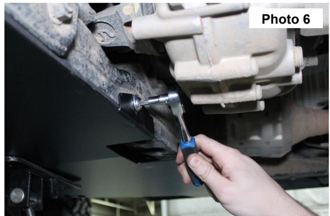
7. Install transfer case skid plate using factory hardware and tighten with a 12mm wrench.
