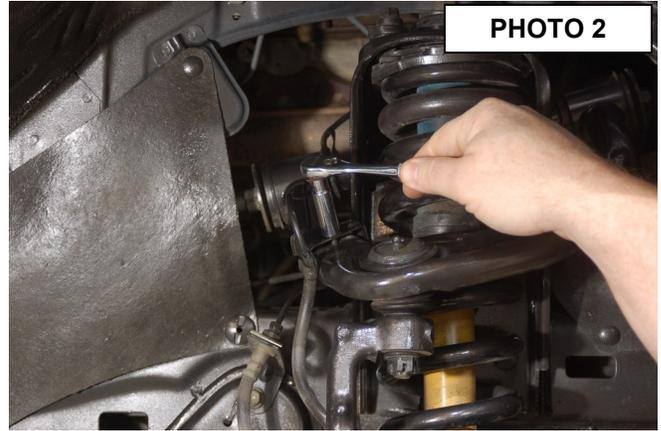
7. Next remove the ABS sensor from the knuckle using a 10mm socket.
