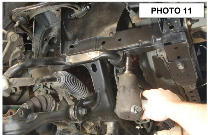
22. Remove the lower control arm with a 21mm socket and wrench. **See Photo 12.**
