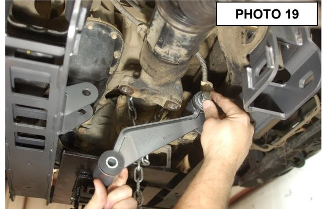
38. Use the factory hardware and a 19mm socket to bolt the passenger side diff to the mounting bracket. Plug the vent tube and the diff actuator back into the diff. Make sure the vent hose and wiring are not rubbing on any moving parts and they have slack in them. Use a 12mm socket to tighten the actuator and top vent tube.
