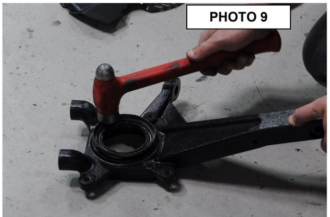
18. Insert the factory hub and dust shield into the Rough Country lifted knuckle and tighten with a 17mm wrench.
