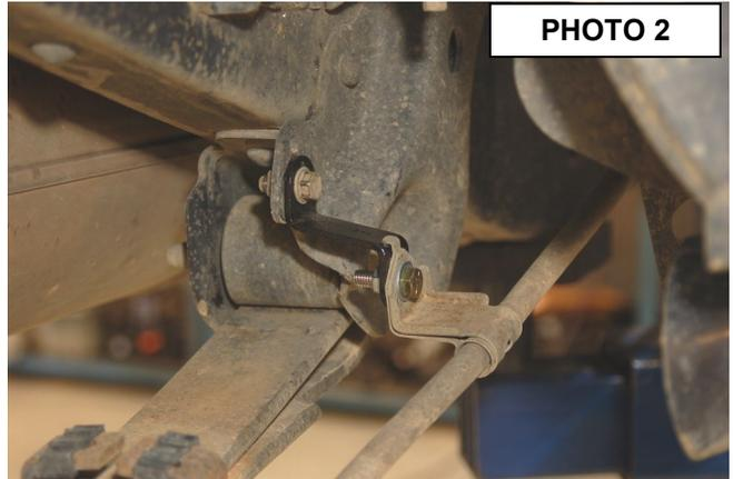
1/4" bolts, washers, and locking nuts to attach the factory mount to the new bracket.
