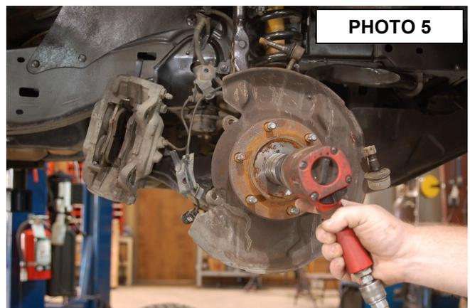
15. On 4WD Models, Use a hammer and punch, carefully remove the CV seal from the factory knuckle. See Photos 6
