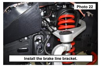
23. Tighten using a 10mm wrench. See Photo 23.
