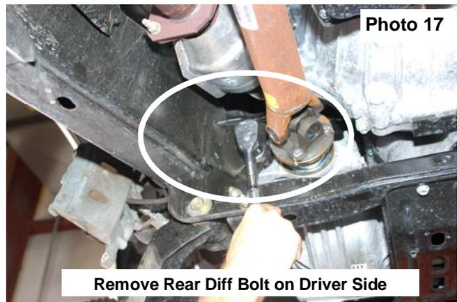
20. Remove the differential vent hose from the top of the differential and lower the differential from the vehicle. (4WD ONLY)
