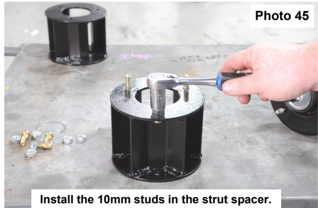
Install the 10mm studs in the strut spacer.
