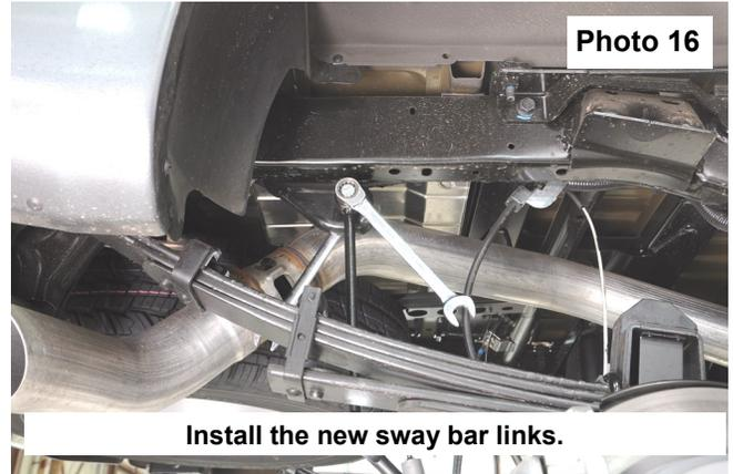
19. Tighten the sway bar links using 18mm and 19mm wrenches. **See Photo 17.**
