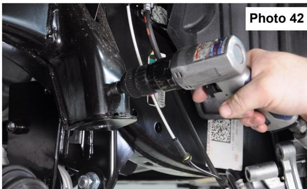
**Drill hole in side of bump stop to 3/4".**
