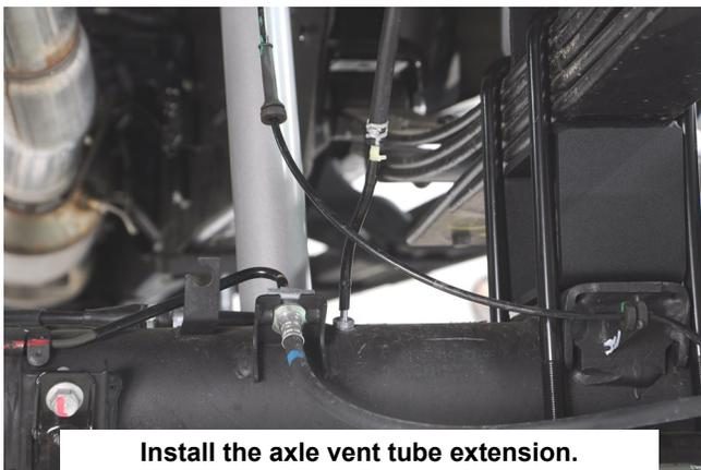
**Install the axle vent tube extension.**
