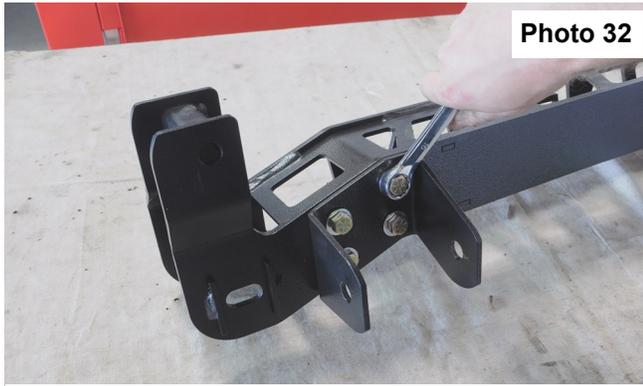
**Install differential drop brackets on front crossmember.**
