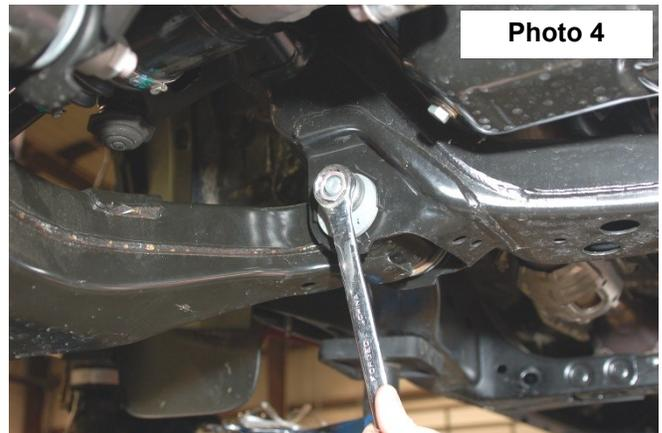
8. Remove the brake line bracket from the knuckle using a 12MM wrench. Retain hardware for reuse.
