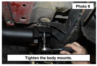
8. Tighten the front and rear body mount bolts using a 5/8 socket. **See Photo 9.**
