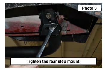
7. Tighten the front and rear step mounts using a 19mm wrench. See Photo 7 and 8.
