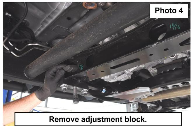
7. Remove the torsion bar adjustment block and factory torsion key. **See Photo 4.**
