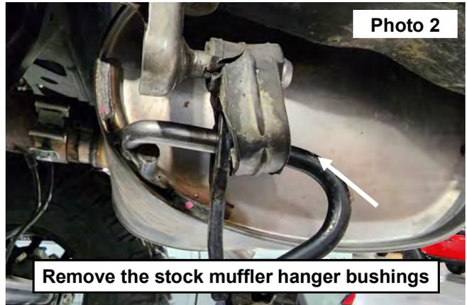
3. Remove the muffler from the vehicle.
