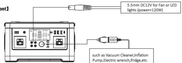
※ **Note:** The 12V DC output voltage is range between 9V~12.6V, maximum output current is 12A. DC output voltage drops while battery capacity drops due to chemical characteristics of the battery. If your appliance is not built-in input voltage stabilizing function, it may shutdown when input voltage is too low, please unplug your device from the unit in time. And please charge the unit in time.
