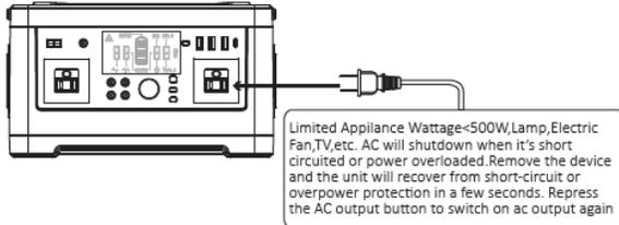
**Warning:** the plug standard and voltage differs according to countries, please make sure the socket standard matches your appliance before using, in case of any dangerous situations.
