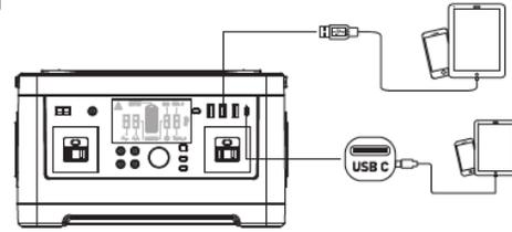
※ Note: When the product is in overloaded or short-circuit protection, please remove the load and USB auto activation
