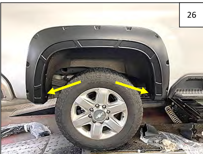
Hold flare on fender. Start 2 factory screws removed in Steps 16 and 18 as shown.
