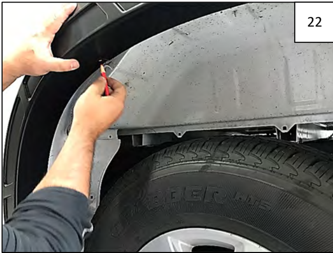
Hold the flare on the fender and mark 5 holes using a grease pencil.
