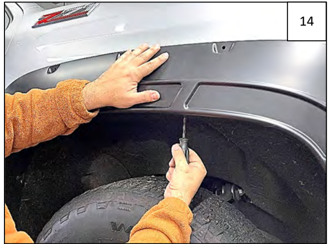
Apply pressure to flare towards vehicle body at each fastening point and tighten all fasteners.
