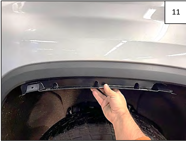
Install Inner Bracket using 2 T15 Torx screws retained in Step 10. Tighten both fasteners.
