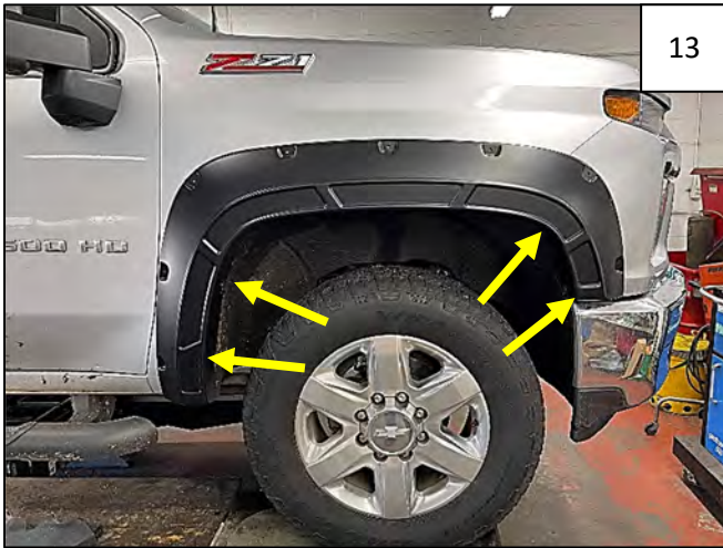
Reinstall 4 factory screws through holes in flare and into holes in fender.
