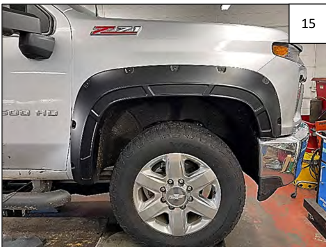
Complete Front Flare Installation.
