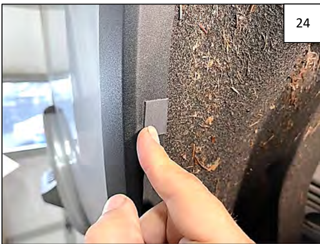
Peel liner from a supplied Foam Tab and center tab over each mark made in Step 22, folding over lip of wheel well.
